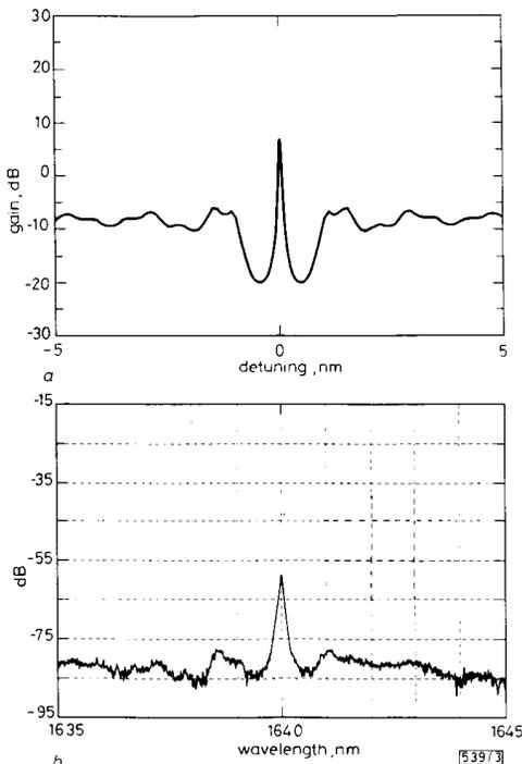
Fig. 3 Calculated and measured output noise spectra of DBR laser with 225  $\mu\text{m}$  long gain section and 360  $\mu\text{m}$  long grating section
