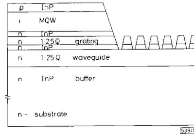
Fig. 1 Growth layer structure of DBR laser
